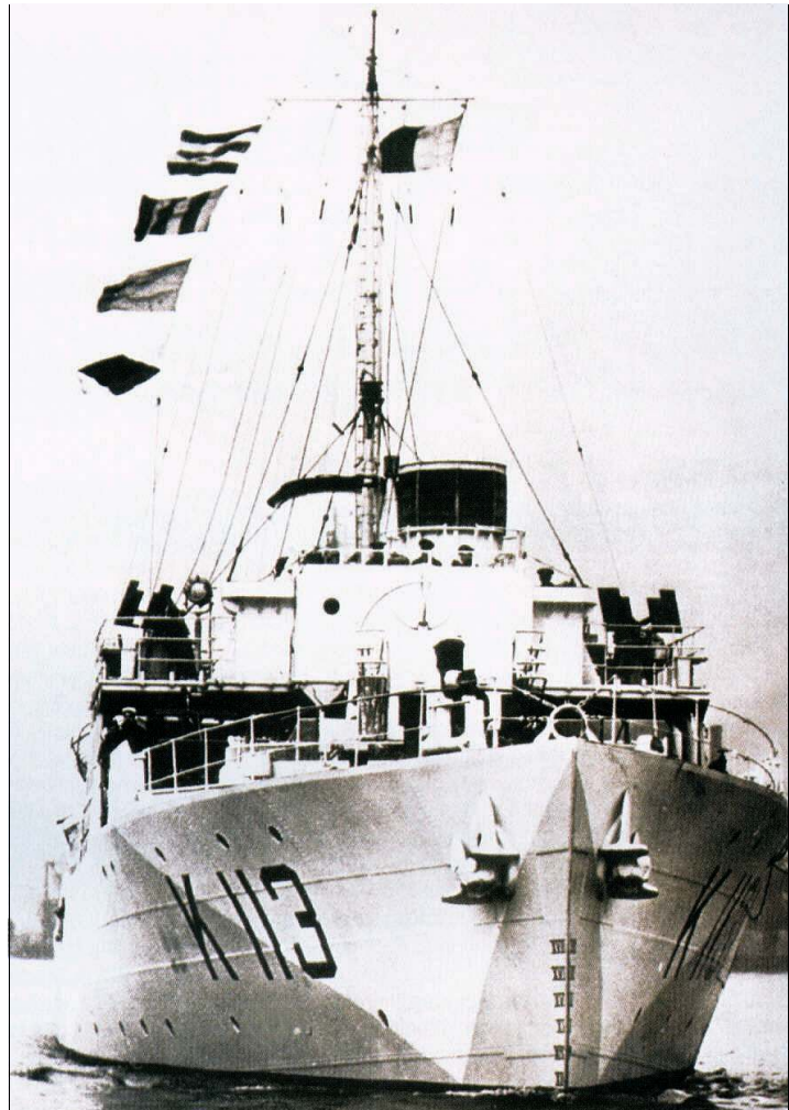
A good view of the bluff bow of the original Flower -class ships. Later vessels would see more flair added to their bows for better seakeeping. Shown is the HMCS Arvida (K-113) early in 1944. Armament would vary from ship to ship largely depending on which area it served. Those operating in European waters generally carried more AA armament than those assigned to convoy duty
